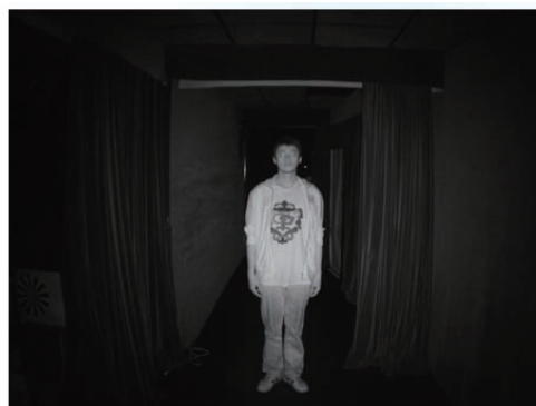
Smart IR enabled; distance: 3M
